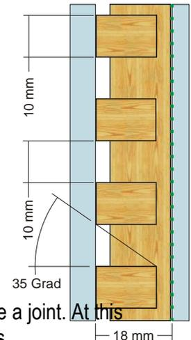
Widths or heights in excess of the maximum lengths specified in the table above require a joint. At this joint it may be possible to see a gap or even an offset between the neighbouring louvres.
